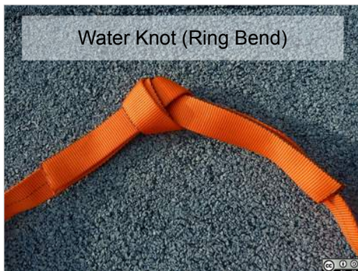
Water Knot – bend to tie in webbing.
