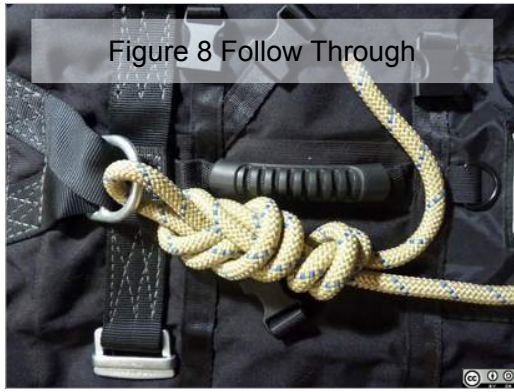
Figure 8 follow through, finished knot
