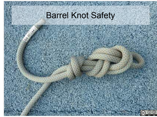
Barrell knot safety (on a figure 8 on a bight).
