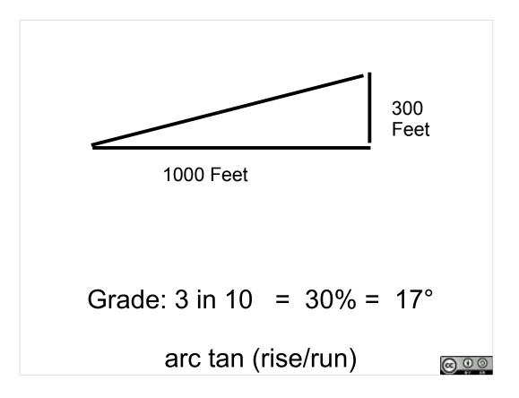
With a calculator we can work out the angle – arc tan of the grade, 17 degrees for a 30% grade.
