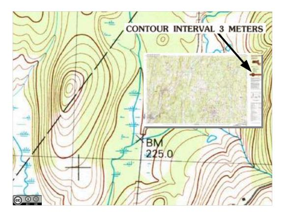
The metadata on the map border can tell us how far apart the contour lines are – what the contour interval is.
