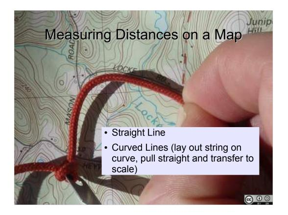
With a ruler or the edge of your compass, you can measure straight line distances on the map easily using the scale.
