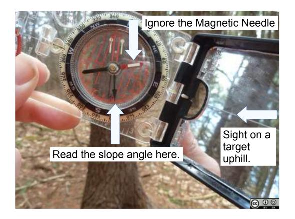
Some compasses have a free hanging needle that allows the compass to be used as an inclinometer – to measure a slope.
