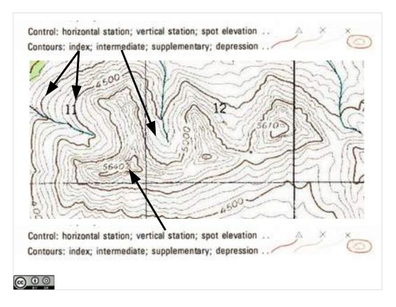
Contour lines are often of two line weights – thick lines with elevations on them (index contour lines), and thin lines without elevations (intermediate contour lines). The contour interval is the (vertical) distance between intermediate (thin) contour lines.
