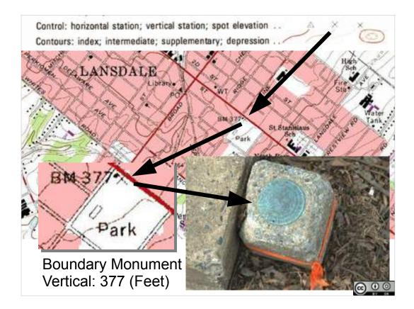
Here is a vertical station, a boundary marker with a surveyed elevation of 377 feet. (Technically, this is a vertical control station, common parlance is "a benchmark").
