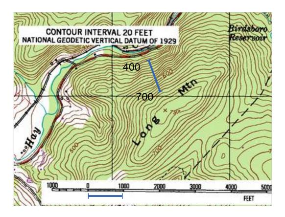
Vertical distance along the blue bar is 300 feet (400 foot contour line to 700 foot contour line)
