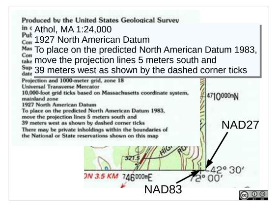
Here is metadata from the border of the Athol, MA 1:25,000 USGS topographic map from 1998. How much difference is there between the grid on the map (NAD27 datum) and WGS84? [39 m west, and 5 m south]
