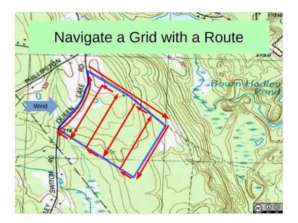
You can create a set of waypoints, then connect those waypoints into a route to navigate a grid of a segment.
