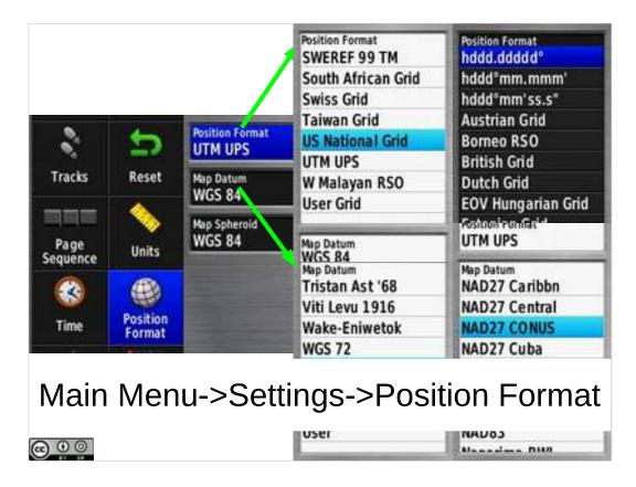
Here's the menu system for a more recent Garmin GPS 62 series GNSS receiver, with position format and datum accessed from a Position Format section on the main menu.
