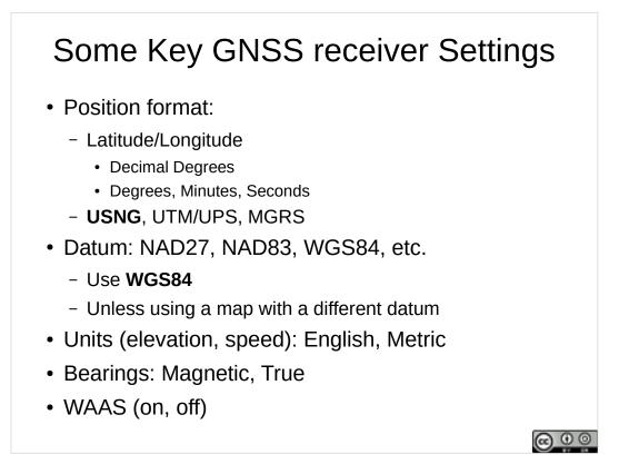
One set of opportunities for **human error** are the GNSS receiver settings. You must be able to locate and change all these settings on GNSS receivers.
