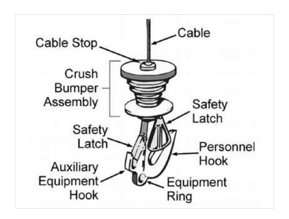
This is a typical helicopter rescue hook. Humans get hooked into the large hook (not the smaller auxiliary equipment hook or the equipment ring).
