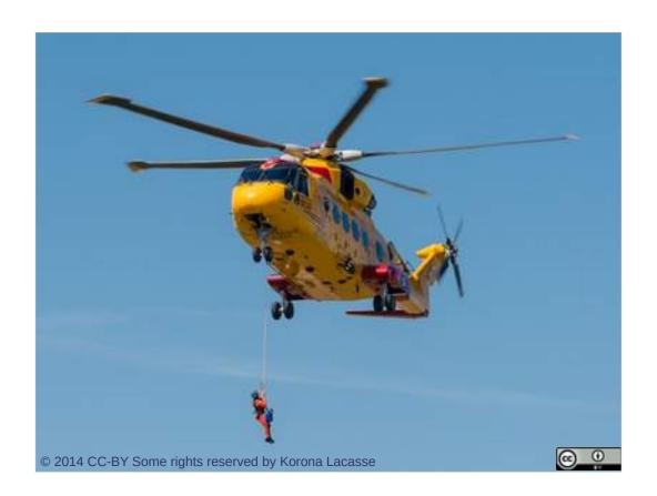
Helicopters with appropriate equipment, certifications and trained crew can perform some rescue operations (vertical hoist between the ground and the helicopter; rarely short haul or long haul).
