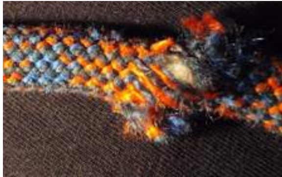
8mm half rope damaged in a leader fall.
