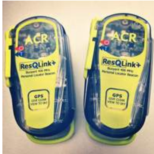
"ACR ResQLink 406MHz Personal Locator Beacon (PLB) with GPS" © 2014 CC Attribution Share Alike Some rights reserved by Tony Webster
