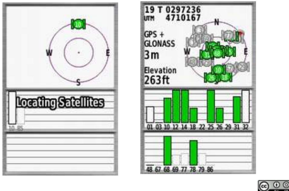
Turn on your GNSS/GPS receiver, it listens to satellites to figure out where it is. This takes time and a good enough view of the satellites in the sky.
