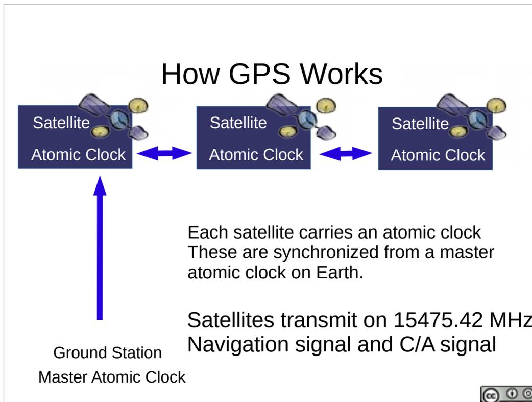
The GPS system is a marvel. It depends on very precisely synchronized atomic clocks carried on each GPS satellite. The satellites transmit a variety of spread spectrum signals in the low microwave bands. The key civilian signals are the Navigation signal and the Coarse/Acquisition signal.
