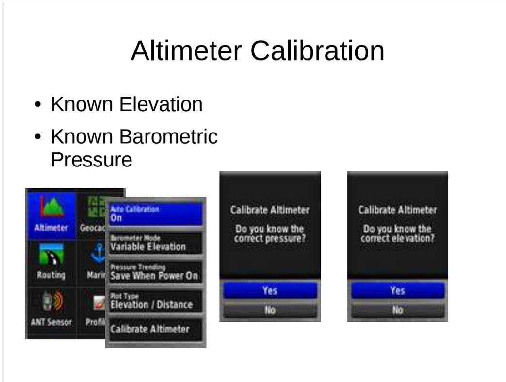
Some GNSS receivers also have an altimeter that can provide a better elevation than GNSS alone (mostly important for mountainous terrain, can also be display barometric pressure trends for weather forecasting).
