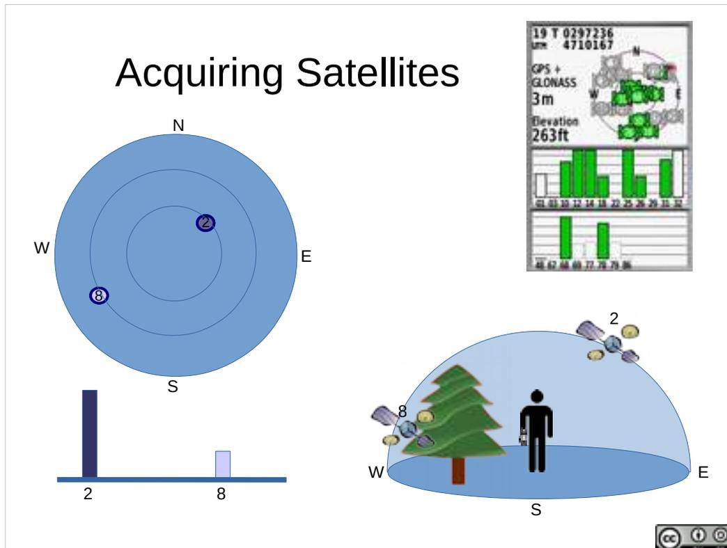
The concentric circles in the display represent the dome of the sky overhead (with North, South, East and West marked). A satellite in the center is right overhead. A satellite near the edge is near the horizon.
