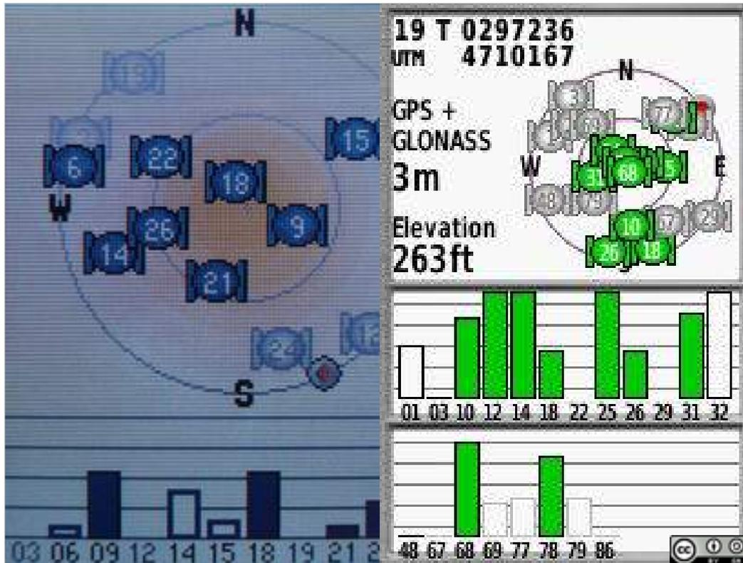
Here's a couple of GNSS receiver's view of what satellites they are currently receiving.
