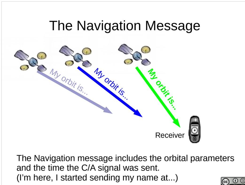
Each satellite also transmits a navigation message containing the information needed to calculate its orbit (and where in its orbit it is) and information needed to determine the exact time that the PRN name was sent.
